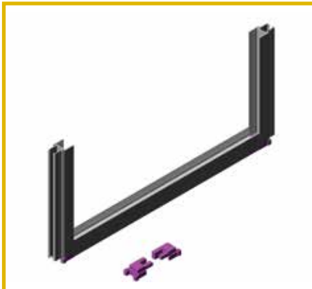
SABİT SİSTEM OLURSA ALT KÖŞE TAKOZU IF IT'S A FIXED SYSTEM, THEN THE BOTTOM CORNER WEDGE.
