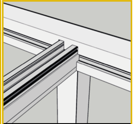
ÇİFTLİ RAY BİRLEŞME DETAYI DOUBLE RAIL INTERCONNECTION DETAIL
